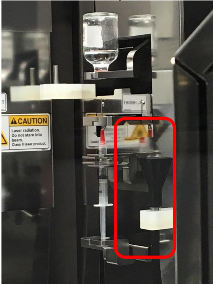
with a discrete particle counter to provide continuous particle monitoring of the compounding cell. The IKFs are located adjacent to the critical sites, and smoke testing is used to demonstrate that they do not interfere with smooth airflow at the critical sites. The particle counters run continuously and send particle count data into the control software which checks the particle level against alert/alarm level settings.
